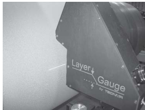
Fig. 9 Online measurement of the bond coat thickness as it is deposited on an industrial strip casting metallic belt
